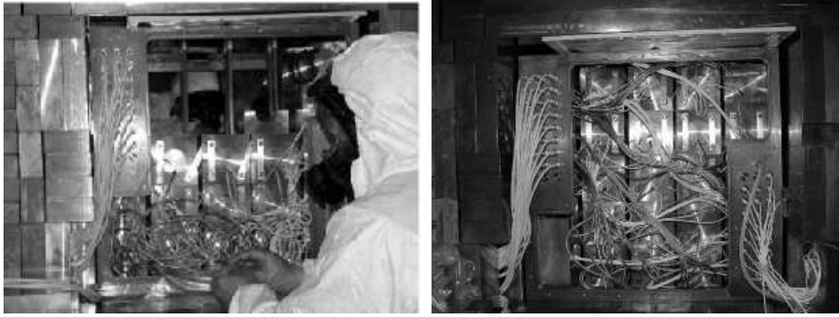
Figure 2.8: Left picture: during the LIBRA detectors installation in HP Nitrogen atmosphere. Right picture: view at end of the detectors installation. All the used materials have been deeply selected for radiopurity (see for example the cables with teflon envelop).
