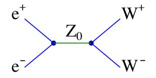
It involves a  $Z_0W^+W^-$  vertex which will suffer radiative corrections proportional to  $\ln m^2$ . Knowing  $\ln m^2$  from a measurement of the  $\rho$ -parameter this value can be inserted in the one-loop calculation of the radiative corrections to the three vertex.
