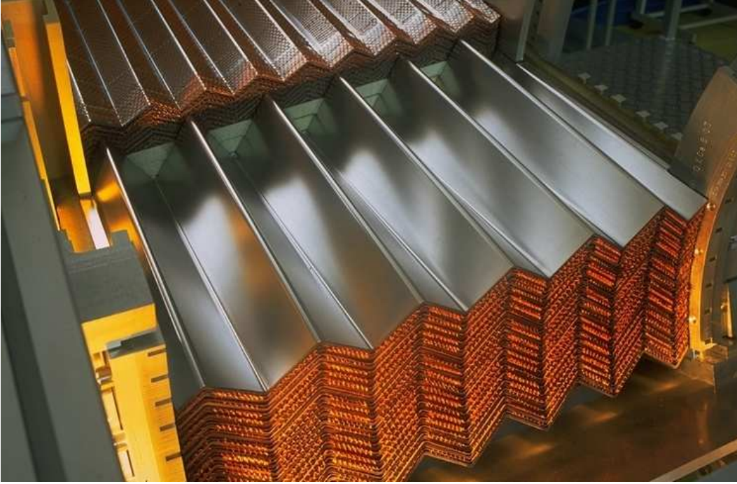
Figure 5. Picture of an electromagnetic end-cap module during stacking, showing the accordion structure of the ATLAS EM calorimeters. The inner wheel is visible in the first plan, with behind a part of the outer wheel. One can notice that the transversal bars of the inner absorbers fill the gap between these two wheels. This light material reduces energy losses in this region. It ensures also an electrical insulation.
