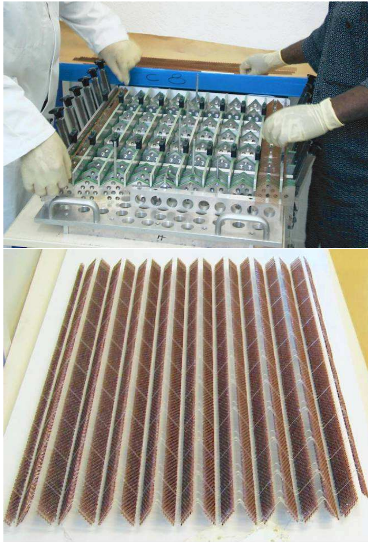
Figure 14. Top: one of the 10 molds for spacer fabrication. Bottom: one of the 10 types of EMEC spacer nets.
