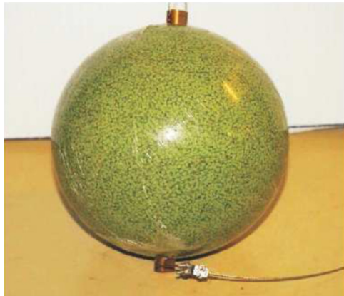
Fig. 11. Picture of the nickel source which was manufactured by CI Kogyo. The ball was made of 6.5 kg of NiO and 3.5 kg of polyethylene. The Cf source was inserted into the center of the ball and held there by a brass rod.
