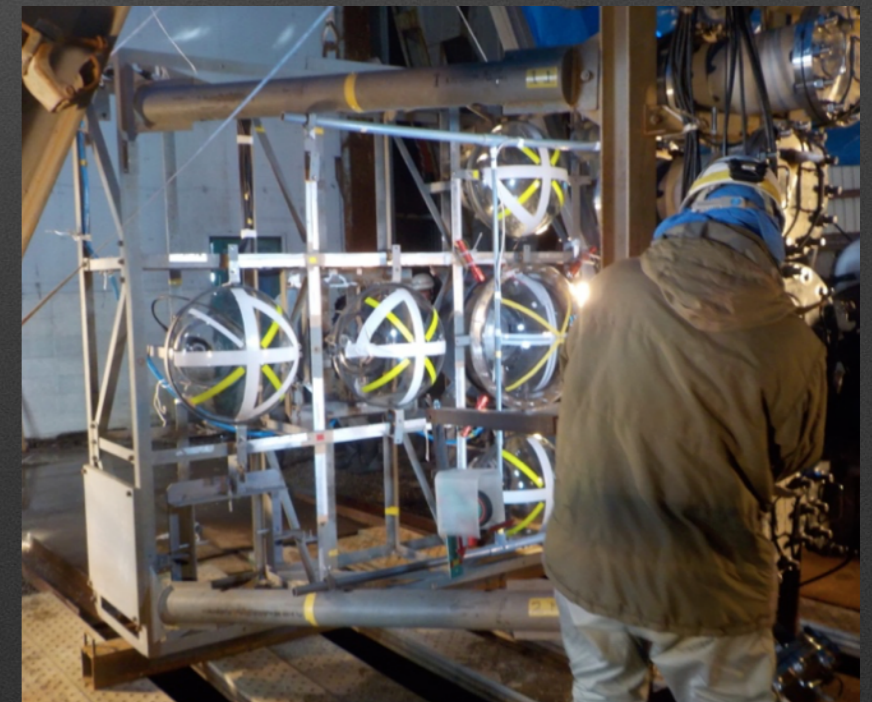
Full cover + witness dummy PMTs on support truss + instrumentation
