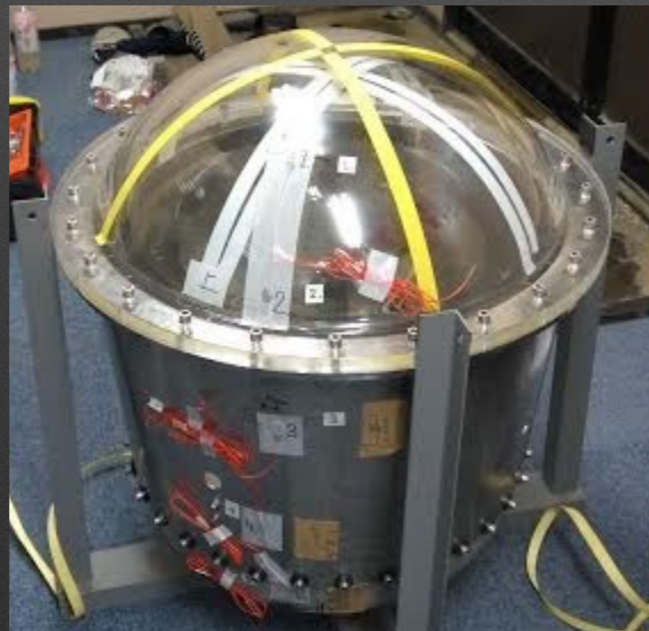
Dummy PMT + acrylic + support hw Strain & pressure gauges
