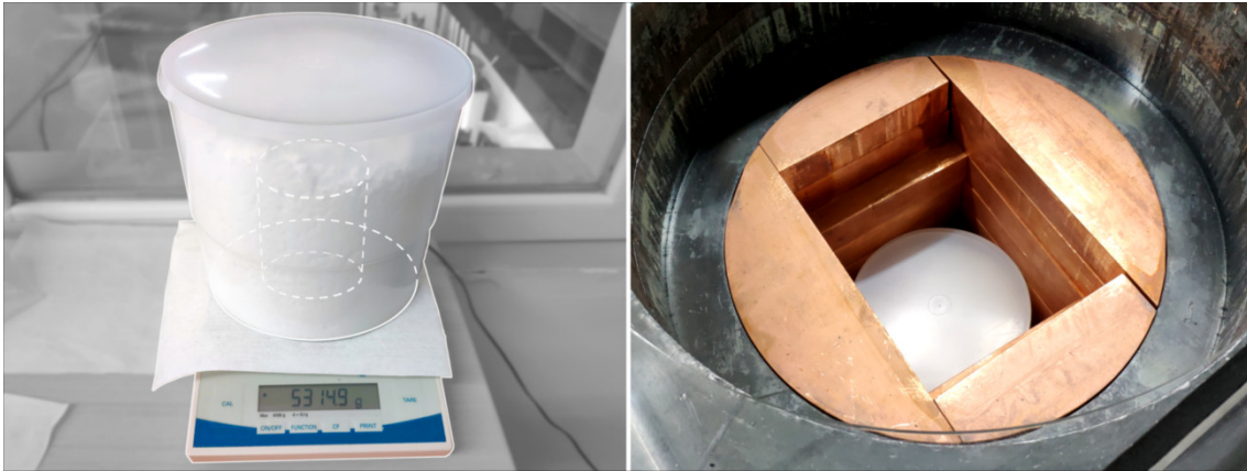
Figure 5.3: On the left, a Marinelli container holding \sim 5 kg of Gd salt about to be measured. Its interior hole is sketched over the photo in white dashed lines. On the right, the container set in the detector, surrounding the HPGe cylinder. Photos took on late 2019 with the permission of the Canfranc Underground Laboratory.
