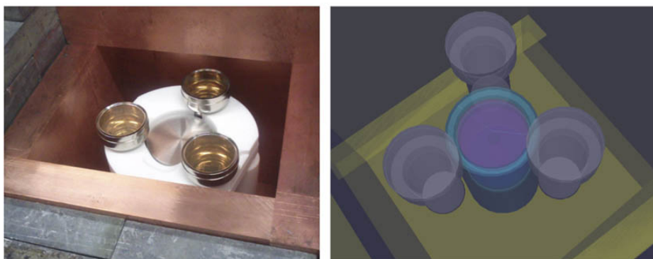
Figure 5.17: Montecarlo simulation of PMTs
