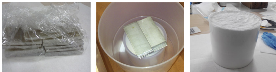
Figure 6.5: Three samples of the water tank of SuperK. Left side, FRP (Fibre-reinforced plastic) sample. Center, Stainless Steel from the water tank. Right side, \text{SiO}_2 candidate to seal a small leak in the water tank
