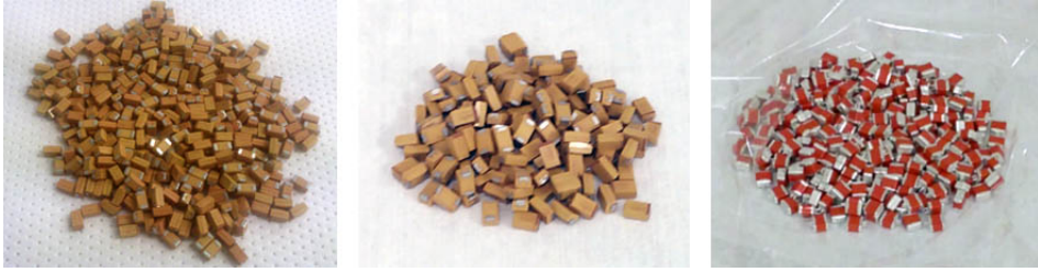
Figure 5.2: Left side, AVX Capacitors 1.5\mu F . Center, AVX Capacitors 4.7\mu F . Right side, Vishay Capacitors
