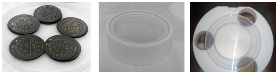
Figure 5.7: Left side, Kapton Substrate. Center, Sapphire Crystals placed in a Teflon support. Right side, Optical Gel
