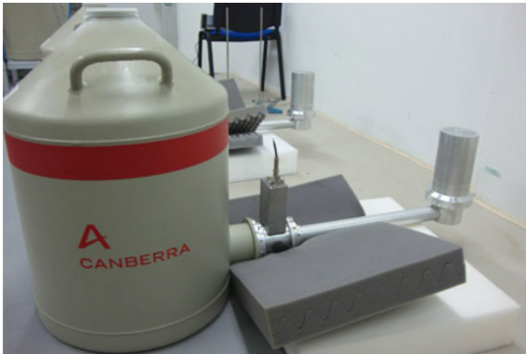
Figure 4.7: View of the HPGe without the shielding
