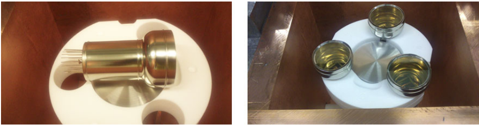
Figure 5.14: Left side, horizontal configuration of the PMTs, with the unit above the detector. Right side, 3 PMTs configuration, with them around the detector.
