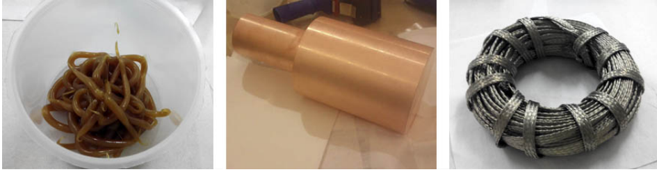
Figure 5.12: Left side, Vacuum Grease. Center, part of the CuA1 sample for HPGe. Right side, CuSn Braid
