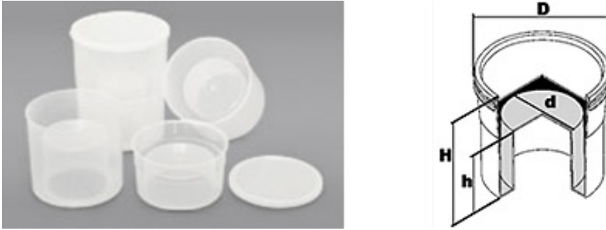
Figure 4.10: Sample of different Marinellis beakers employed at LSC for radiopurity measurements
