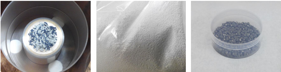
Figure 5.28: Left side, 10GOhm Ohmcraft Resistors. Center, Teflon Powder. Right side, Getter pills
