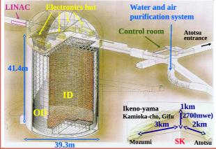
Go further with high efficiency neutron tagging: SuperK-Gd
