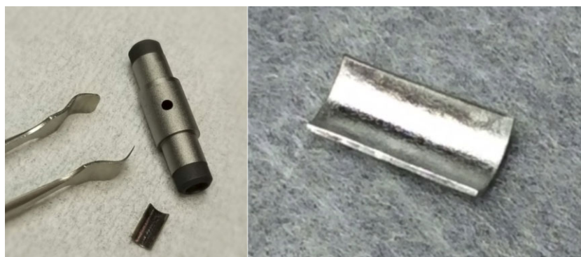
Fig. 3. Left: HR cuvette and Ta platform after formation, ready to be inserted into the cuvette. Right: Close-up view of the platform.
