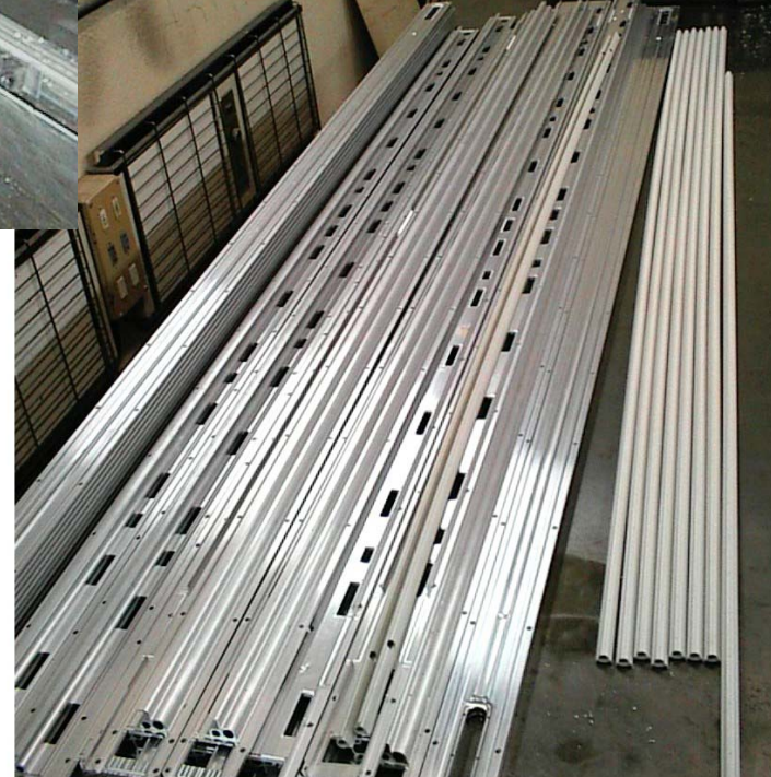
Machining of chamber frames at CIEMAT mechanical workshops
