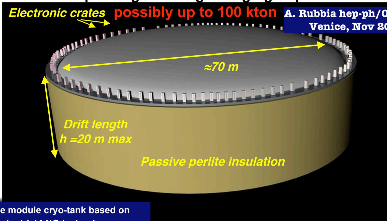
Single module cryo-tank based on industrial LNG technology
