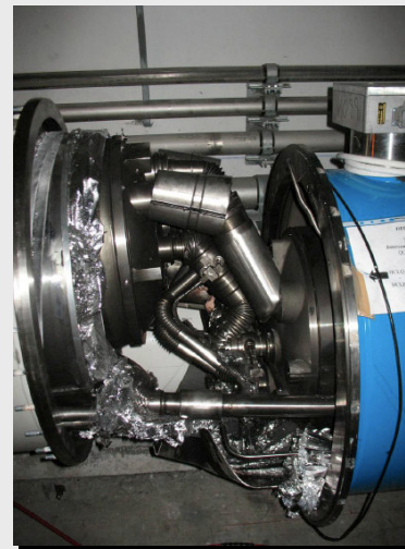
2 most severely damaged interconnects
