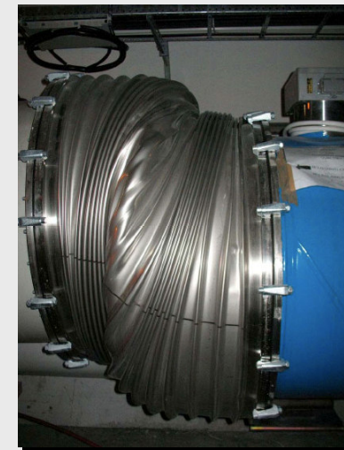
2 most severely damaged interconnects
